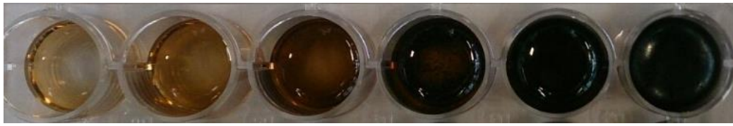
Figure 2. A photograph of a 24-well plate showing the change in colour of the alkaline dopamine solutions over 6 h, 12 h, 24 h, 48 h, 72 h, and 96 h, shown from left to right, respectively.
