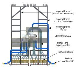
Figure 5.28: Front view of an IT detector station.
