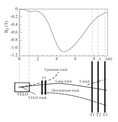
Figure 3.6: Distribution of the magnetic field and the labels given to the various types of track observed across the LHCb tracking detector [24].
