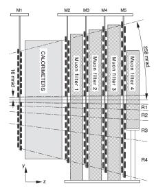
Figure 3.11: The LHCb muon chambers positioned at the extreme downstream part of the detector [24].
