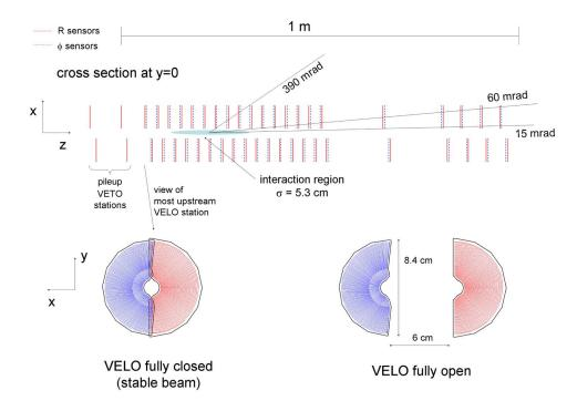
Figure 3.3: Projection of VELO in the y-z plane showing the pile-up veto system upstream and the spacing of the R and  $\Phi$  sensors [24, fig. 5.1, p16]
