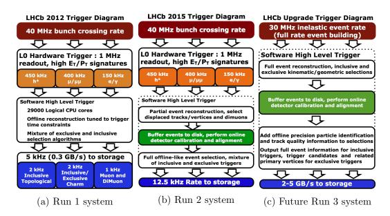
Figure 3.13: Trigger systems between Run 1 and future Run 3 where the hardware L0 will be removed and full event reconstruction will occur at the software level [39].
