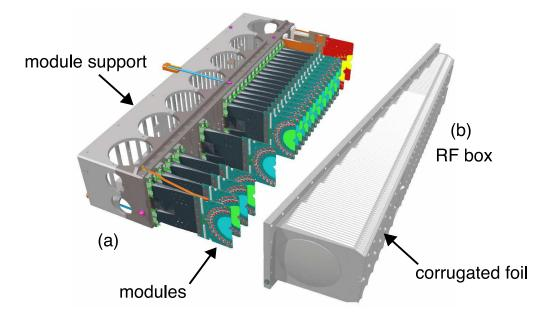
Figure 3.4: View of the VELO showing the surrounding RF foil and movement machinery [24].
