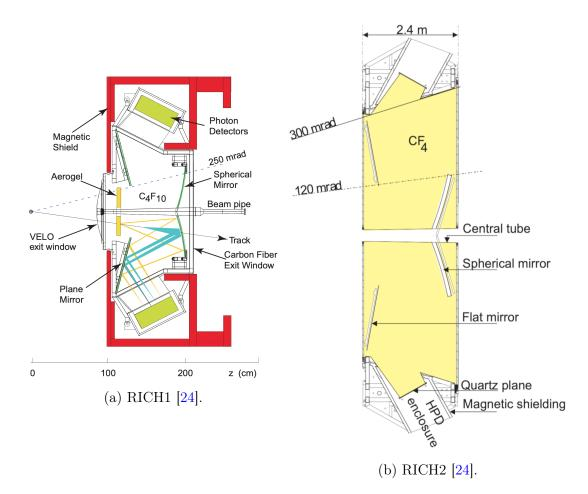
Figure 3.10: The two RICH subdetectors within LHCb situated downstream of the VELO and T1–T3 tracking stations respectively.
