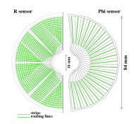
Figure 3.5: Cross section of one R- $\Phi$  station showing the orientation of wiring [27].
