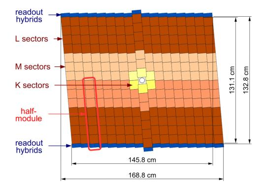
Figure 3.7: Cross section of the Tracker Turicensis (TT) showing the four layers of silicon strips [24].
