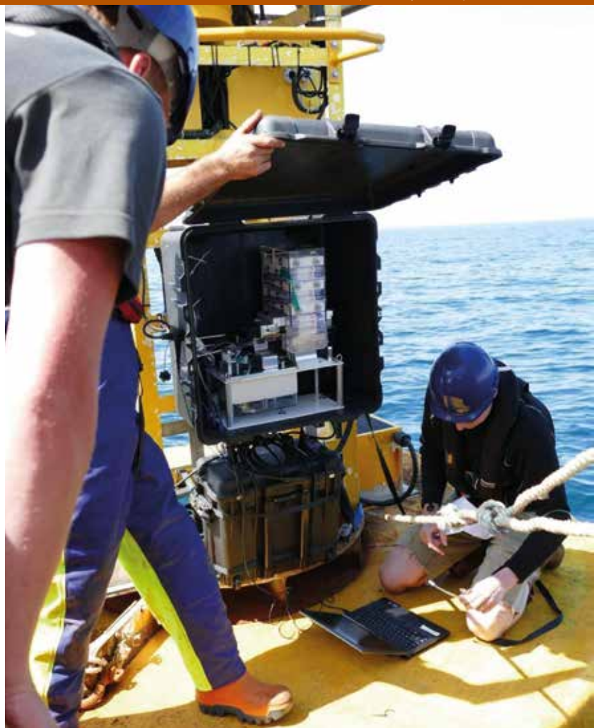
Fig. 1. MAPS Marine Autonomous Plankton Sampler on the long-term buoy L4 of the Western Channel Observatory, English Channel. James Fishwick, Plymouth Marine Laboratory
