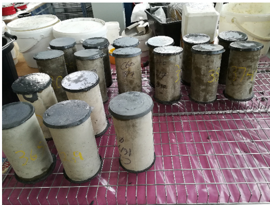
Fig. 3. Cylindrical concrete samples capped with sulphur.
