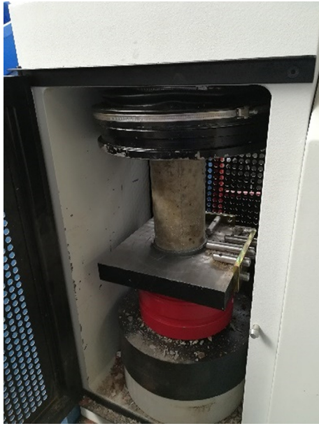
Fig. 2. Concrete compression testing machine.
