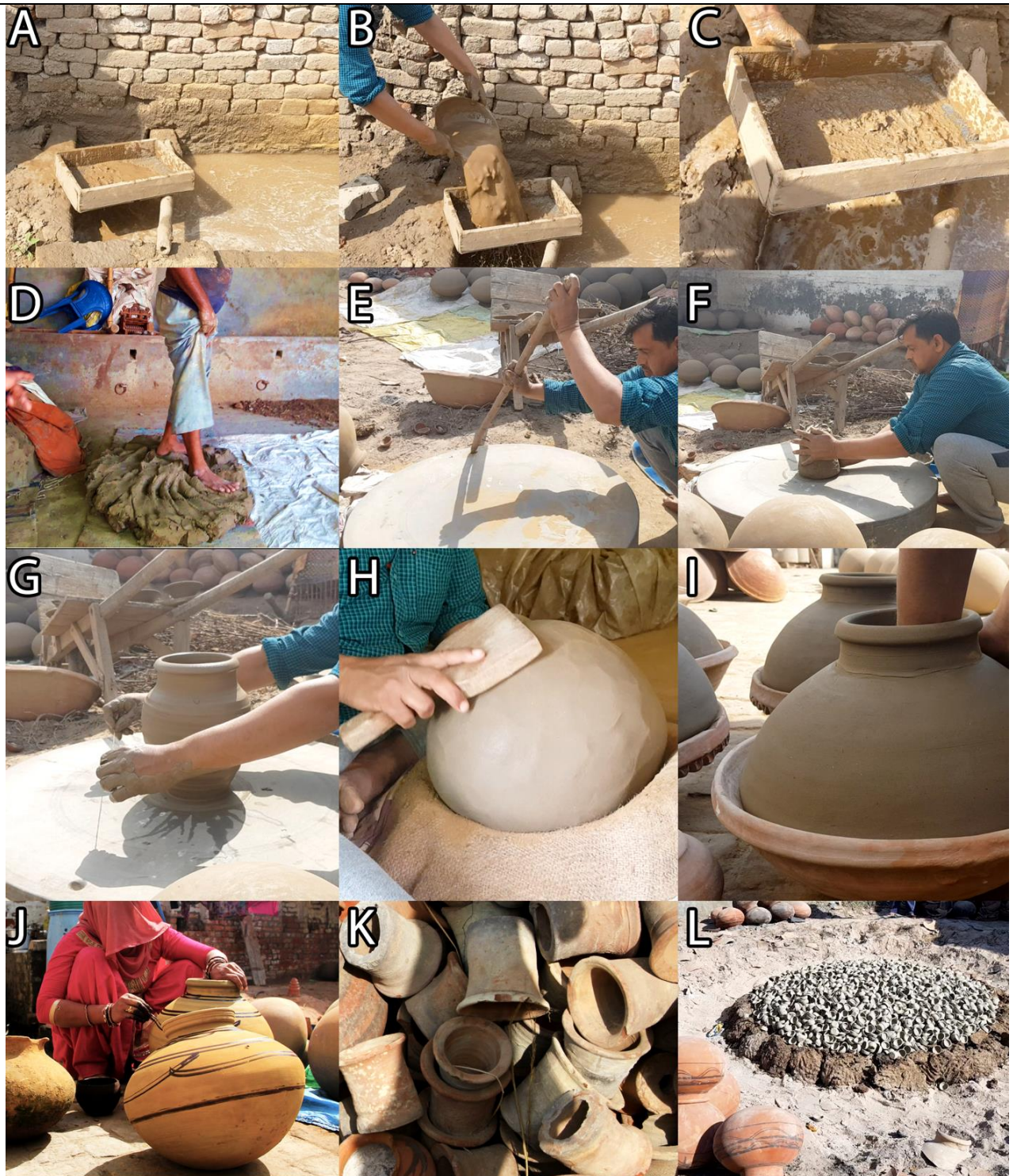
Figure 5.2 Sequence of actions for producing ceramic vessels, including clay cleaning and processing (A-D), setting the potter's wheel in motion and forming vessels (E-I), decorating (J), and firing tools and places (K-L).
