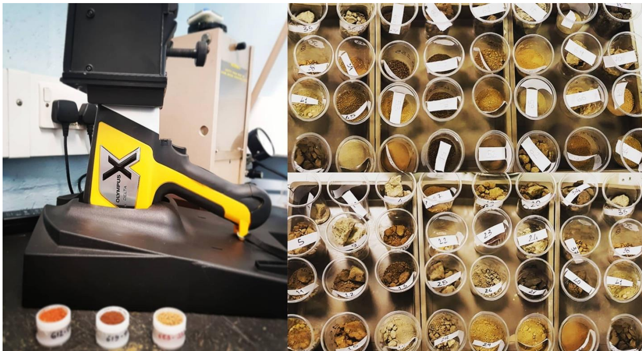
Figure 4.5 Left: pXRF Olympus Innox-X Delta Premium analyser used for processing powder samples and three XRF sample cups or cuvettes of loose powder. Right: dried samples of clay rich deposits from MSD-I trench XK2.
