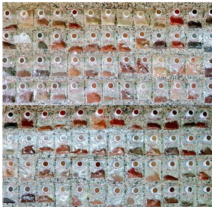
Figure 4.6 Ceramic powder samples from MDS I and cuvettes of loose powder for pXRF Olympus Innox-X Delta Premium hand-held device.
