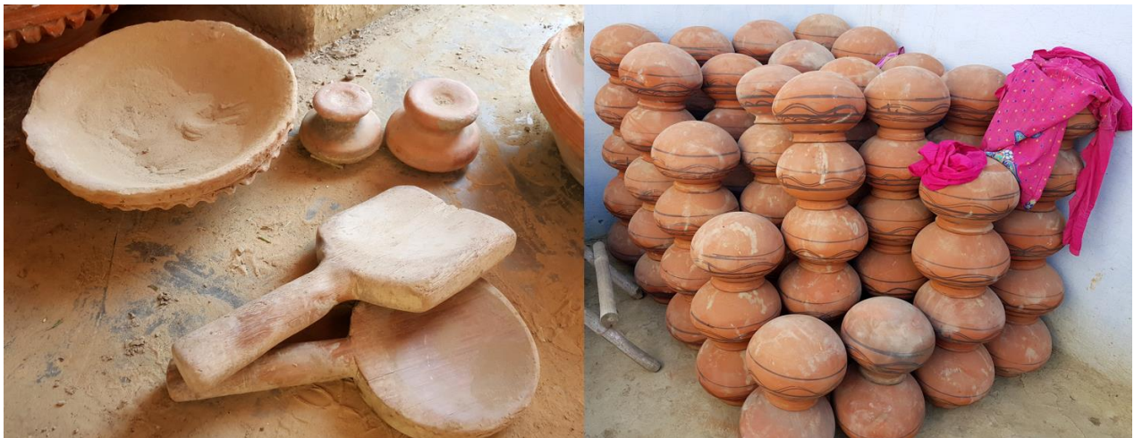
Figure 5.3 Workshop at Masudpur. Left: Paddle-and-anvil and bowl of mica-rich sand; right: finished globular jars.
