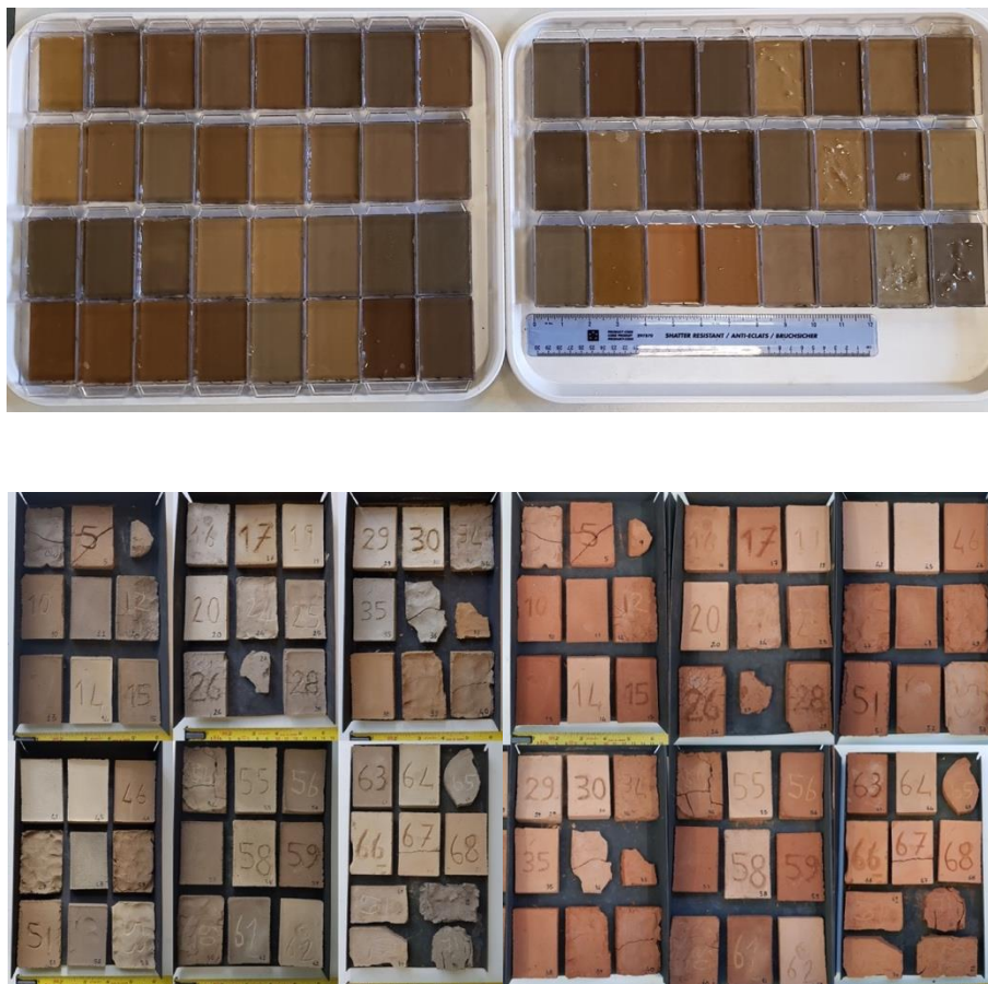
Figure 4.8 Formed briquettes (above), and dried and fired briquettes (below). See Appendix A, table A4 for description of 73 CSR samples.
