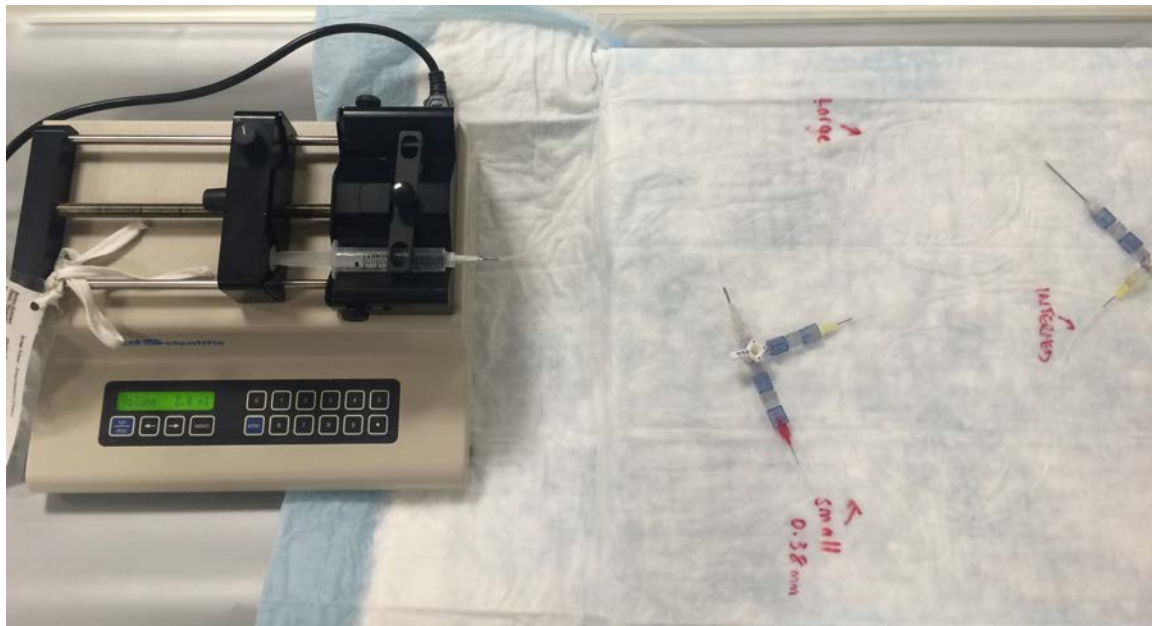
Figure 3.1: Set up of Harvard pump and tubing (large, intermediate and small diameters) to simulate trials for development of initial 4D injection protocol
