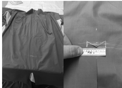
The opening is marked with chalk and cut in.
