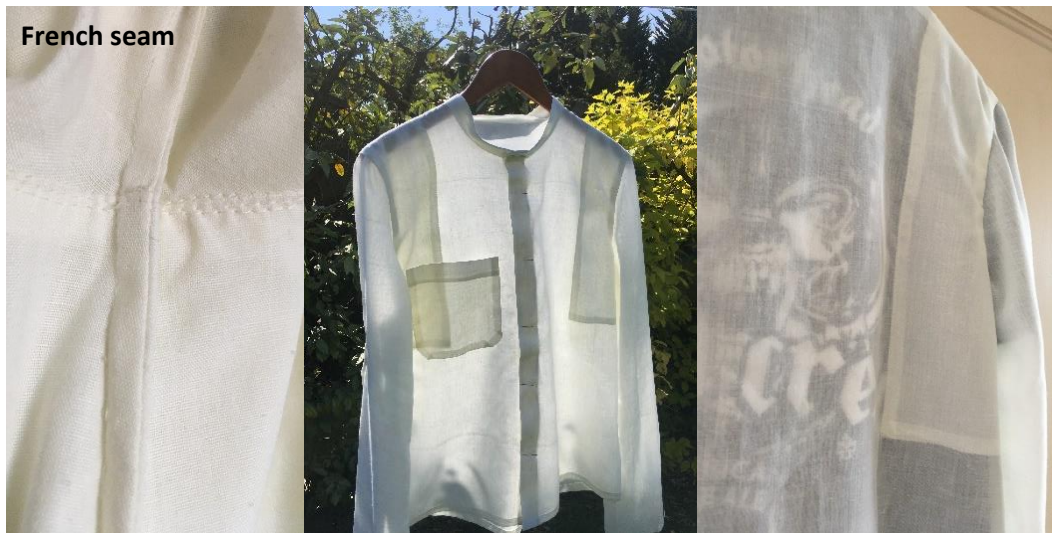
Figure 5.4.6. Mandarin shirt showing, French seaming, construction and layering.
