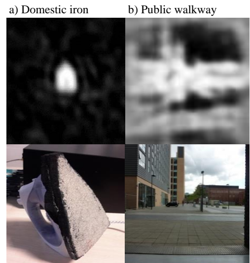
FIGURE 2. Images measured using a 32-channel 22 GHz aperture synthesis imager of: a) an absorber covered domestic iron at 57^\circ\text{C} against an ambient temperature ( 23^\circ\text{C} ) background [22] b) an outdoor public walkway [20], white being radiometrically ‘hot’.
