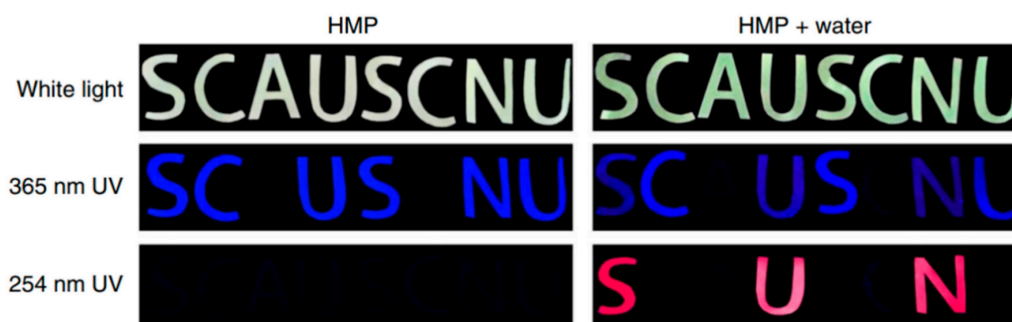
Figure 11. Proof-of-concept security feature made by applying hydrophobic C-dots via marker pen, with and without the addition of water and illuminated under different kinds of light. Reproduced from reference [31], Nature Communications; published by Nature Research, 2019.
