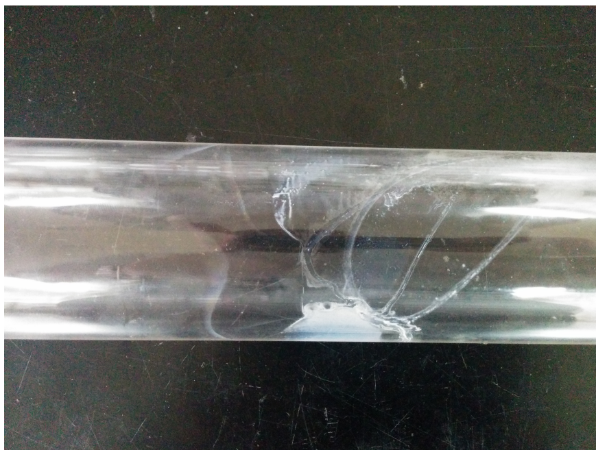
Figure 4: Fused quartz tube of Cs volatilisation rig, shows signs of etching after repeated CsOH volatilisation experiments
