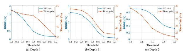
FIGURE 6. Impact of the model threshold on BD rate and time gain
