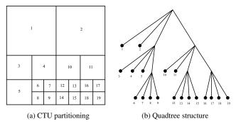
**FIGURE 2.** Sample partitioning structure of a CTU and the corresponding quadtree structure.
