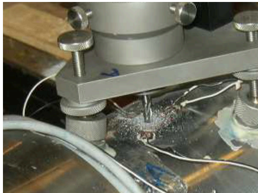
Fig. 2 – Drilling head VISHAY RS-200 and detailed view of the axle drilling
