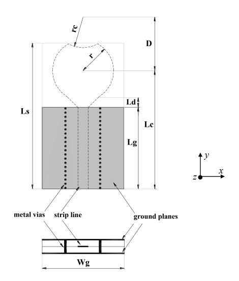
Fig.1. Geometry of the Dual-layer UWB antenna
