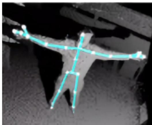
Figure 6. Example skeleton representation obtained from Microsoft Kinect v2 (overlaid on the depth image). The skeleton consists of 25 joints (shown as white circles), here connected with light blue lines for better visualization.
