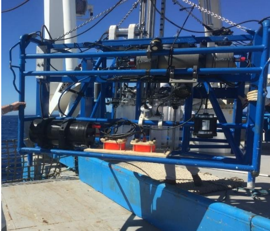
Figure 2.6: The Instrumented Corer Platform (ICP) ready to be deployed.
