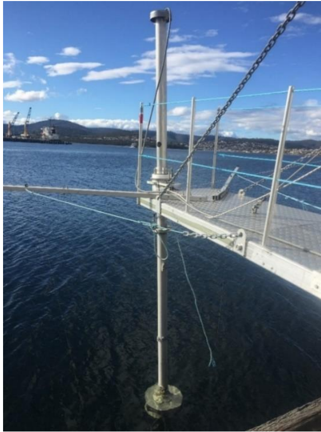
Figure 3.6: An illustration of the experiment set up. A downward-facing transducer was positioned on the platform and connected to the Simrad EK80 software via a cable. A calibration sphere was suspended below the transducer, controlled by three monofilament lines attached to fishing reels.
