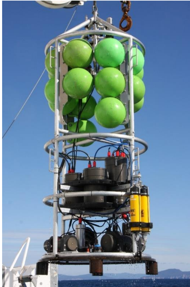
Figure 2.8: A Profiling Langrangian Acoustic Optical System ready to be deployed.
