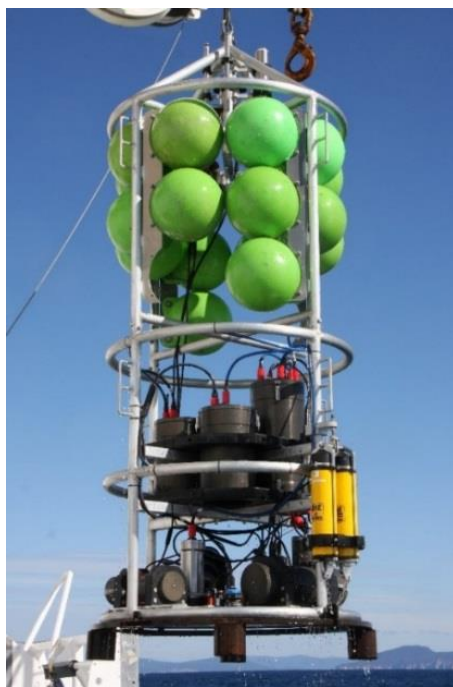
Figure 7.1: The PLAOS ready to be deployed. The platform carried two broadband and a narrowband echosounder, two optical cameras, a video recorder and two optical strobes. The buoys (green) on top allow the platform to maintain the motion.
