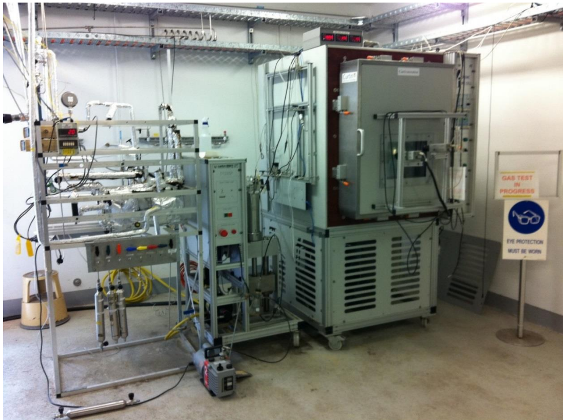
Figure 1.14: PVT cell capable of hydrate testing at high-pressures.
