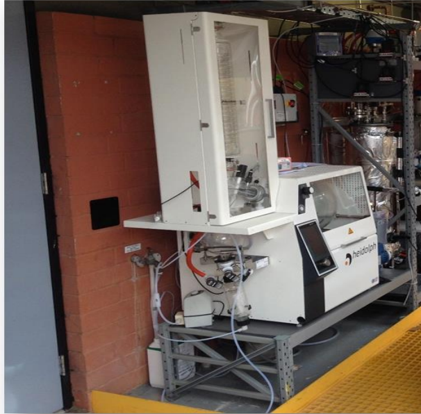
Figure 1.13: MEG reclamation unit (rotary evaporator) at the MEG pilot plant.
