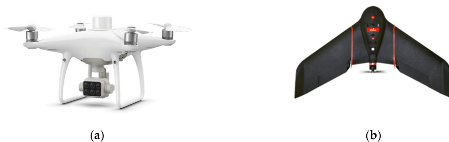
Figure 2. Types of drones based on aerodynamic flight principles. DJI P4 Multispectral ( https://www.dji.com/p4-multispectral/specs ), a multi-rotor drone (a); senseFly eBee SQ ( https://www.sensefly.com/drone/ebee-sq-agriculture-drone/ ), a fixed-wing drone (b).
