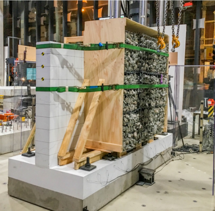
Figure 4.28 Typical set-up of cushion protective layer
