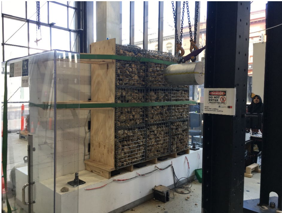
Figure 4.30 Typical set-up of cushion protective layer
