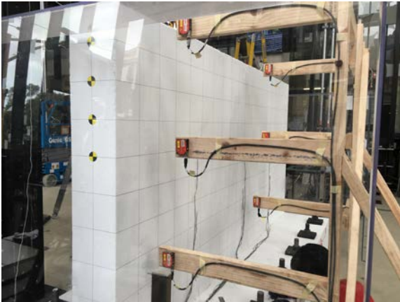
Figure 4.21 Photographs showing laser sensors attached to the timber frame
