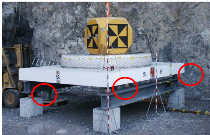
Figure 2.27 - Load-cell arrangement in Schellenberg, Volkwein [16]
