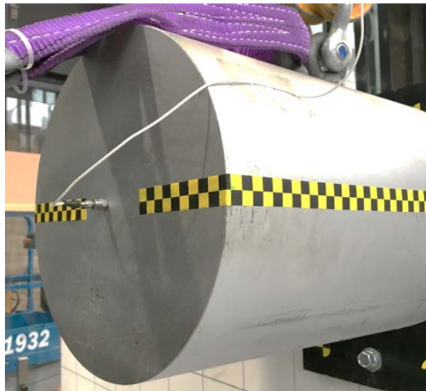
Figure 4.23 Photographs showing the accelerometer sensor attached to 280 kg impactor
