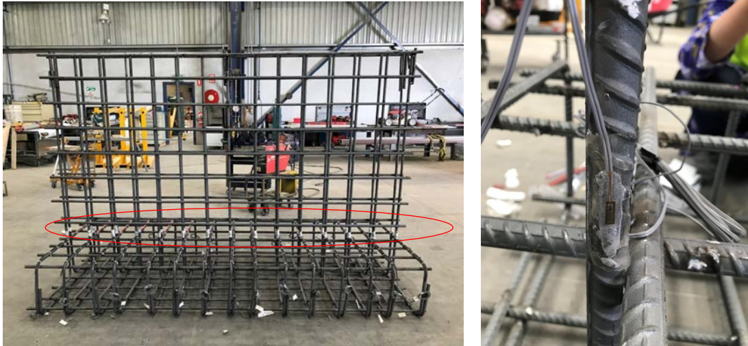
Figure 4.17 Photographs of strain gauges on reinforcement bar -specimen 1
