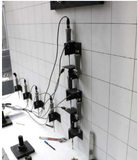
Figure 4.20 Photograph of LVDTs at the front of the wall
