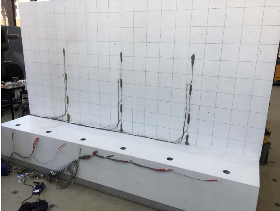
Figure 4.19 Photograph of a strain gauge on concrete surface – specimen 2
