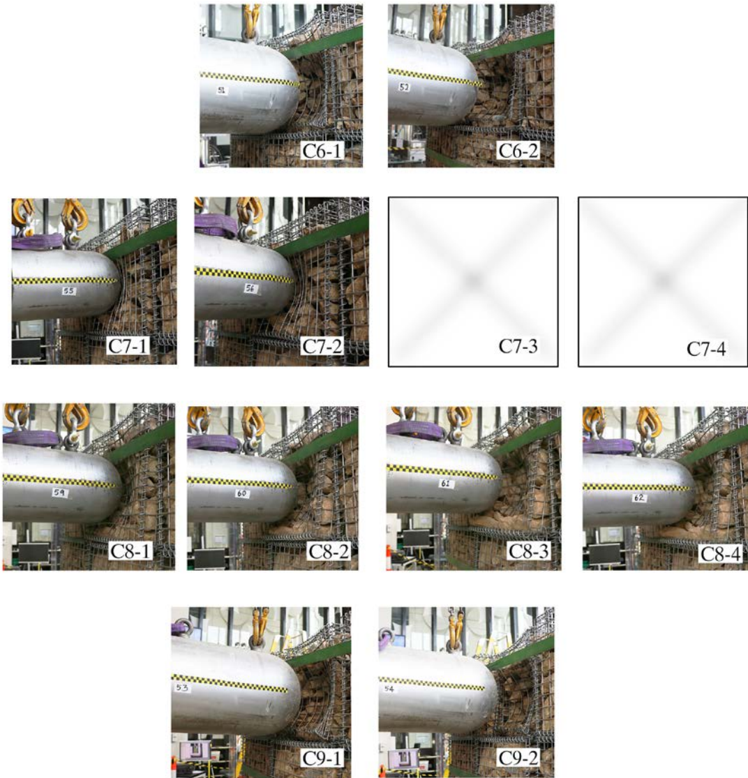
Figure 4.43 Damage to the gabion cushion following the impact – Test Series C
