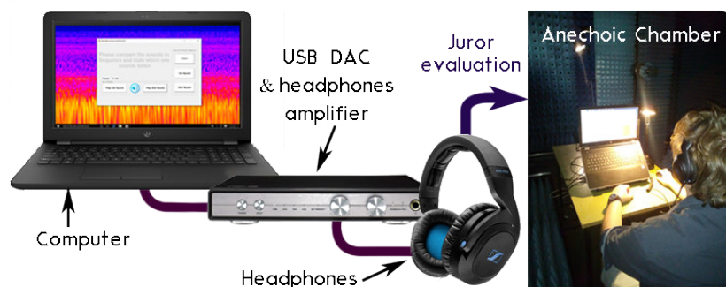
Figure 5.1.1: Jury evaluation test setup showing (left) computer, Xonar Essence DAC and headphone setup and (right) jury evaluation tests being conducted
