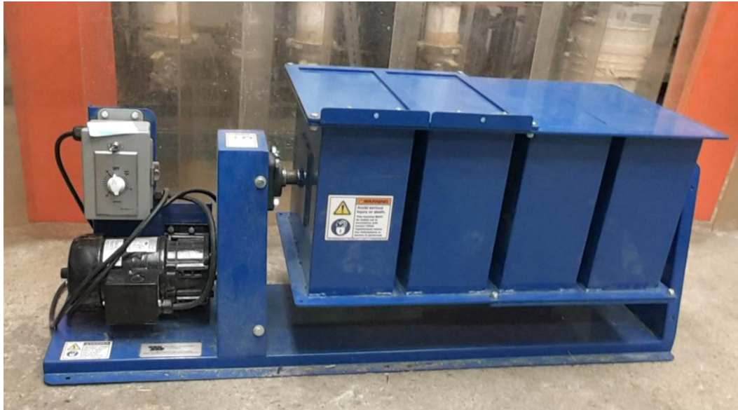
Figure S7.6: Lab-scale Seedburo® pellet durability tester with four dust-tight compartments
