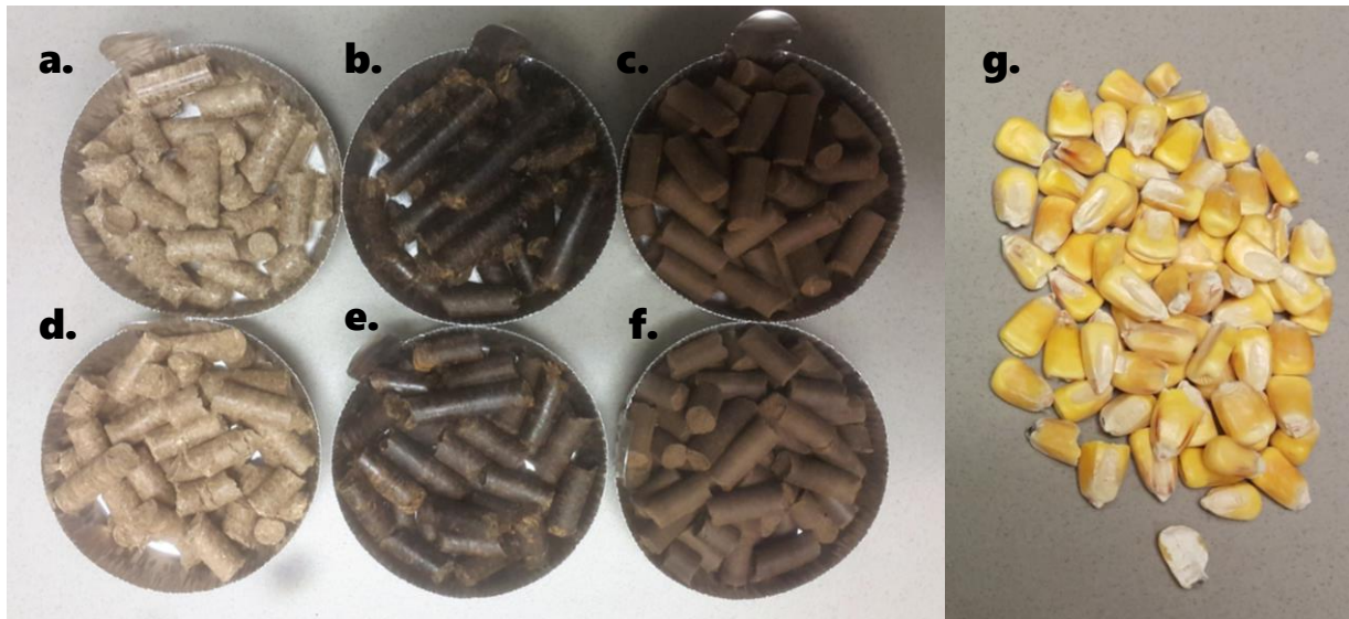
Figure 7.2: Illustration of the untreated, AFEX TM pretreated, StEx pretreated SCB and CLM pellets and corn grains recovered from a commercial 1G ethanol production mill. (a) Untreated SCB, (b) AFEX TM -SCM, (c) StEx-SCB, (d) Untreated CLM, (e) AFEX TM -CLM, (f) StEx-CLM, (g) corn grains
