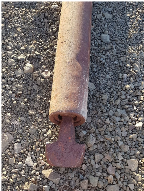
Figure 24: The bottom of a bailer. Source: Private archive of Albertus Steenkamp of the farm Klipbank, Carnarvon.
