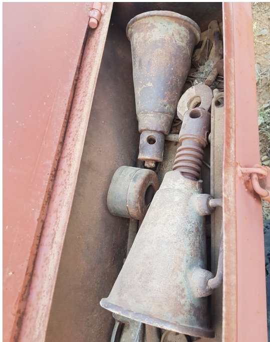
Figure 29: A bellows used to heat the drill tip. The tip is heated and hammered to sharpen it and create the desired diameter. Source: Private archive of Albertus Steenkamp of the farm Klipbank, Carnarvon.
