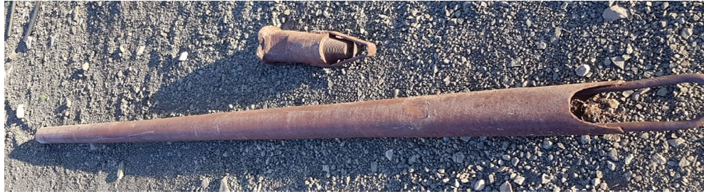
Figure 23: A dill tip (top) and bailer (bottom). Source: Private archive of Albertus Steenkamp of the farm Klipbank, Carnarvon.
