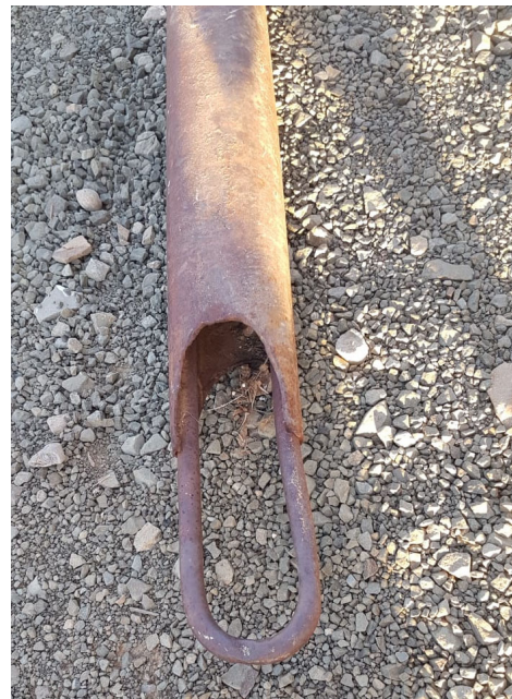
Figure 25: The top of a bailer. Source: Private archive of Albertus Steenkamp of the farm Klipbank, Carnarvon.
