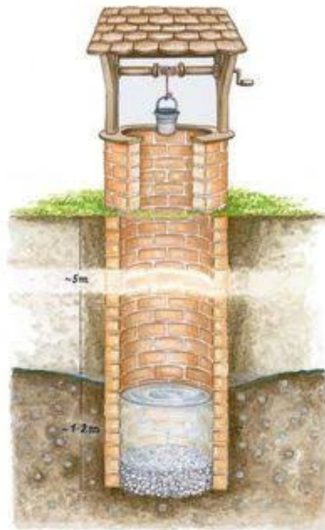
Figure 16: An illustration of a rolput , or hand crank well. Source: J. Olley, Human- and Animal-Powered Water Lifters for Irrigation Practical Action , The Schumacher Centre, Rugby, UK, 2008, p. 56.
