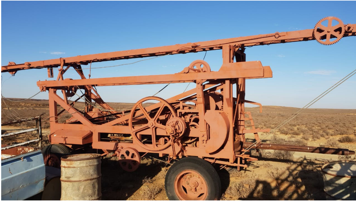
Figure 21: A Jumper drill. The top beam is raised vertically for the cable to droop over when the machine is in use. Source: Private archive of Albertus Steenkamp of the farm Klipbank, Carnarvon.
