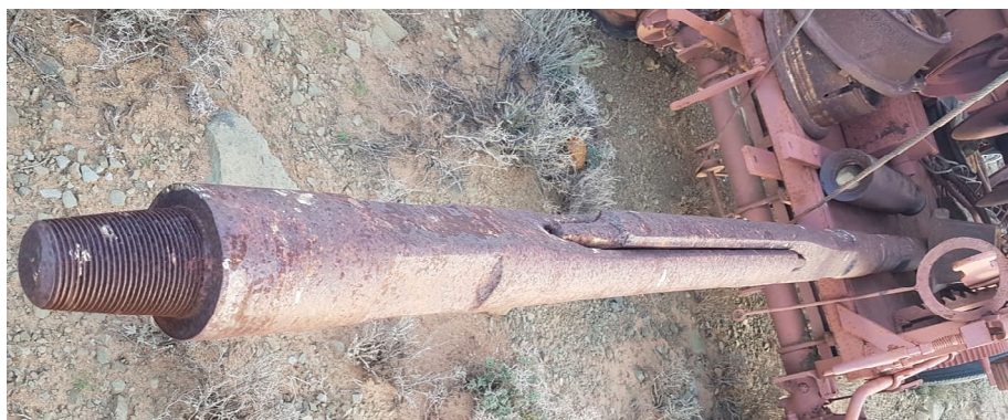
Figure 26: Attachable jumper drill bits used to lower the drill tip into the ground as it drills. Source: Private archive of Albertus Steenkamp of the farm Klipbank, Carnarvon.
