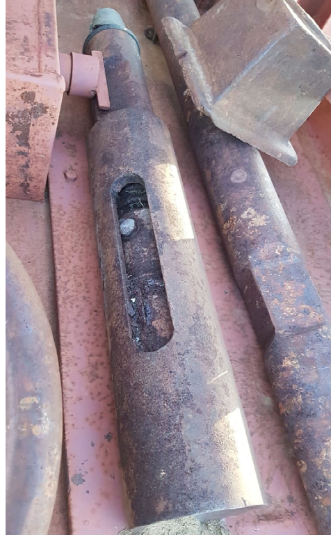
Figure 28: Drill tip catcher, used to attach the drill bit. Source: Private archive of Albertus Steenkamp of the farm Klipbank, Carnarvon.
