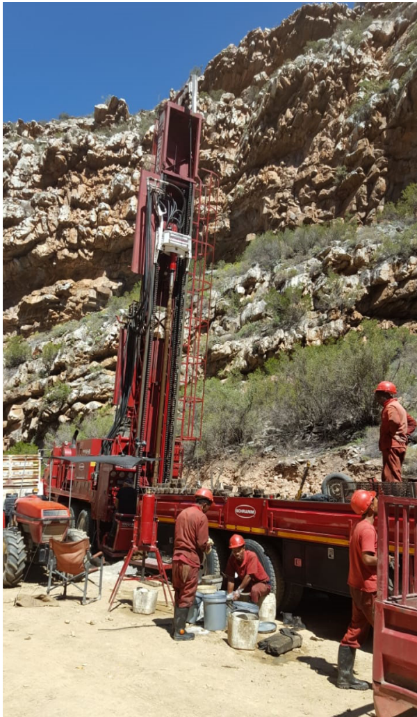
Figure 31: An air-pressure drill. Source: Private archive of Dirk Steyn of the farm De Oude Muur, Montagu.
