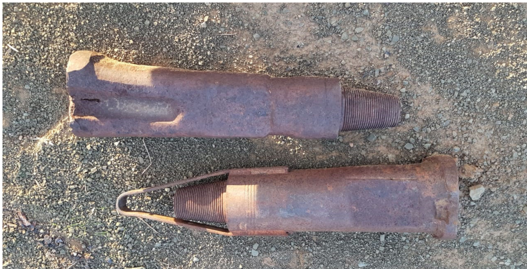
Figure 22: Two drill tips. The bottom tip has been modified to break rocks more effectively. Source: Private archive of Albertus Steenkamp of the farm Klipbank, Carnarvon.
