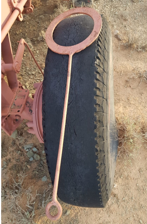
Figure 27: Measuring instrument used to ensure the borehole remains the same diameter throughout. Source: Private archive of Albertus Steenkamp of the farm Klipbank, Carnarvon.
