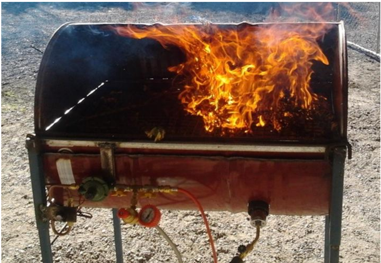
Figure 1-2 The device used to measure the shoot flammability of plants.
