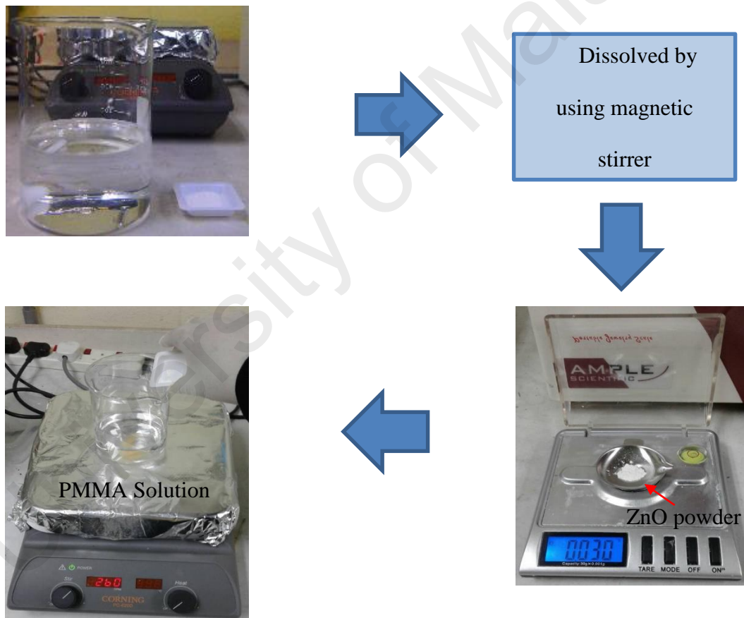
Figure 4.2: Fabricate ZnO PMMA thin film
