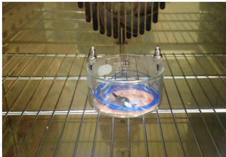
Figure 4.7: Dry oven technique with few-layer of \text{Bi}_2\text{Te}_3 drop on the surface of fiber ferrule.
