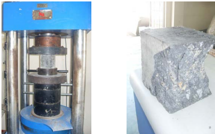
Fig. 4. Compressive strength test setup.
