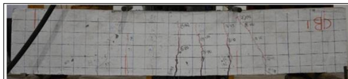
Figure 4. Crack pattern of CB
