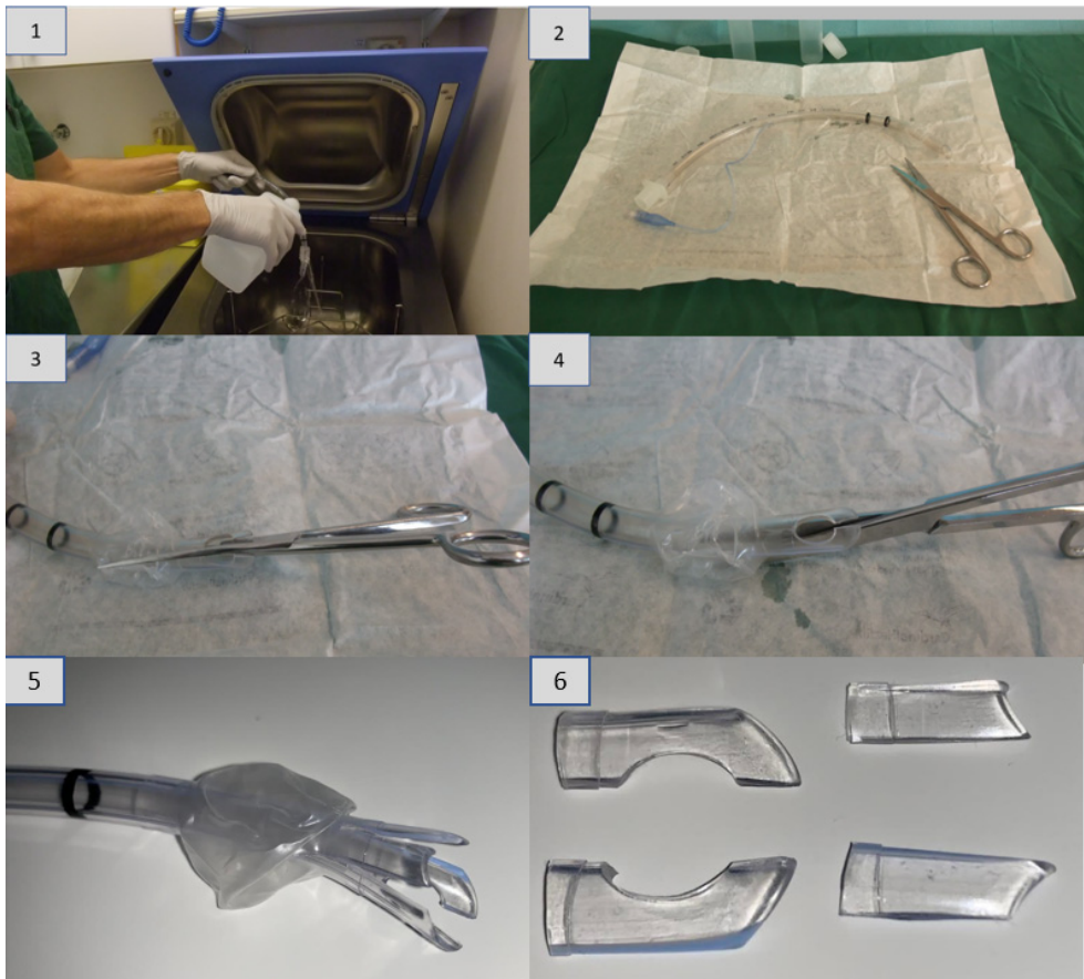
Figure 5. Processing of endotracheal tubes (ETTs): (1) each ETT was rinsed with sterile saline, on the inside and outside, to eliminate excess mucus; (2–6) photographs showing how ETTs were cut for scanning electron microscopy (two pieces) and microbial culture (two pieces). Photos by Bengt Klarin and Hulda Thorarinsdottir.
