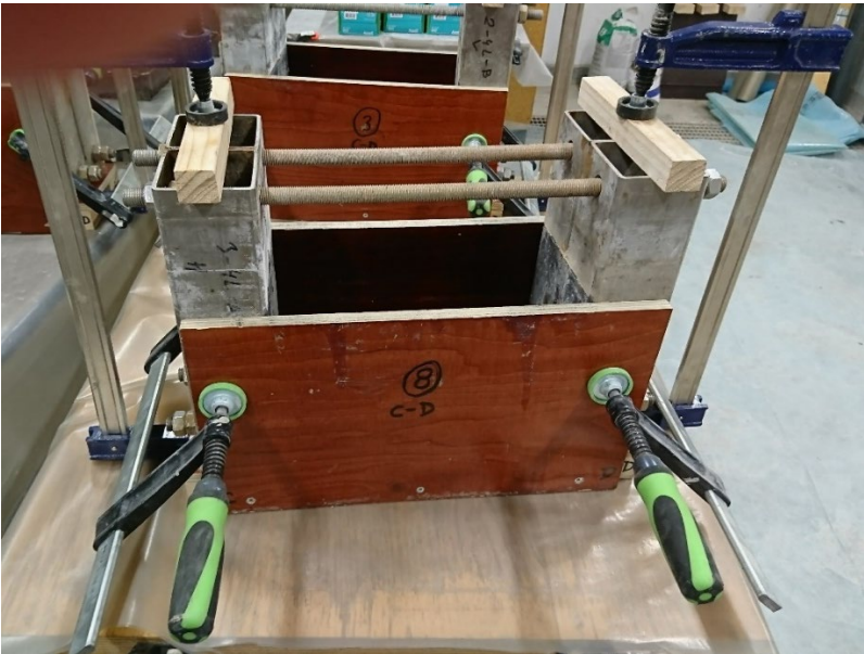
Figure 2. The formwork for the concrete beams.
