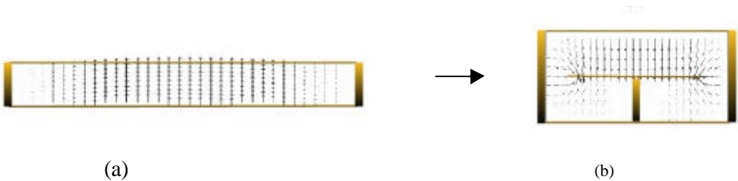
Fig. 1. Cross-sectional view of a standard waveguide (a) and folded waveguide (b)
