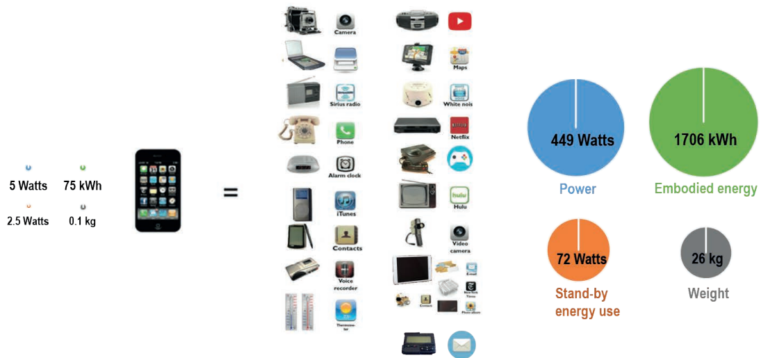
Figure 23. The rapid progress of information and telecommunication technologies could be an indication of the path-breaking potential of next-generation digital technologies and their clustering in new activities and associated behaviors. A smartphone needs between 2.2 Watts in standby to some 5 Watts in use, while the numerous devices portrayed in the figure that it replaces need up to a hundred times more power. There is about a factor 25 reduction of embedded energy required to produce the devices and a proportional reduction in emissions. Bundling of services from various devices in the smartphone can be regarded as an example of the power of the Digital Revolution and its huge potential to increase resource efficiencies through new technologies and behaviors. Source: based on data in Grubler et al. (2018) and visualization of Tupy (2012), Graphic courtesy of Nuno Bento, cfr. TWI2050 (2019), Figure 20.
