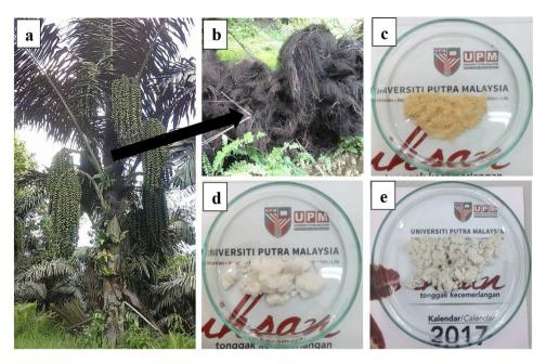
Fig. 1 – Photographs of (a) the sugar palm tree, (b) raw sugar palm fibres, (c) bleached fibres, (d) alkali-treated fibres, and (e) refined fibres.
