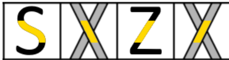
Figure 2: The letter S next to a s-cross, and the letter Z next to a z-cross. The relevant sections of each are highlighted.
