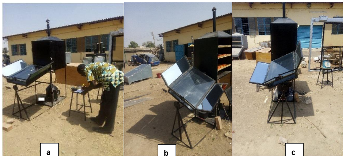
Figure 3: Pictorial (real) views of the FPC (a) facing the sun at noon time (b) facing east before noon time (c) facing west after noon time.
