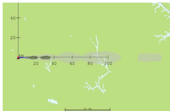
Figure 76: HPAC 4.04 Dose Rate Contour for 1kt Surface Burst with 10kph Constant Wind
