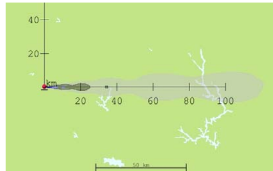
Figure 63: HPAC 4.04 Dose Rate Contour for 1kt Surface Burst with No Rain at 12 Hours
