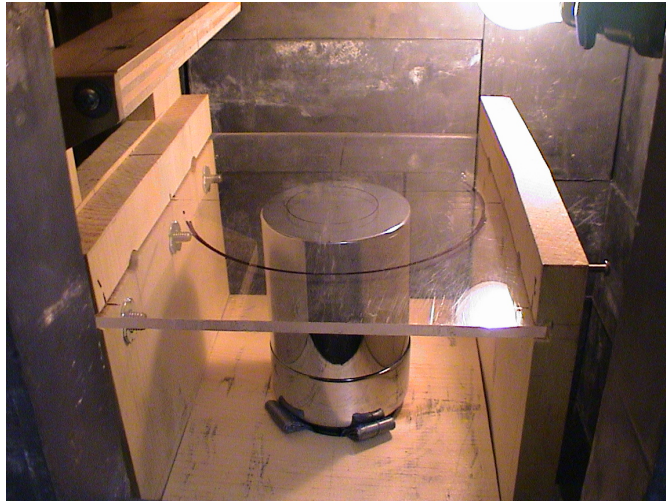
Figure 68. NaI(Tl) in detector housing inside lead cave
