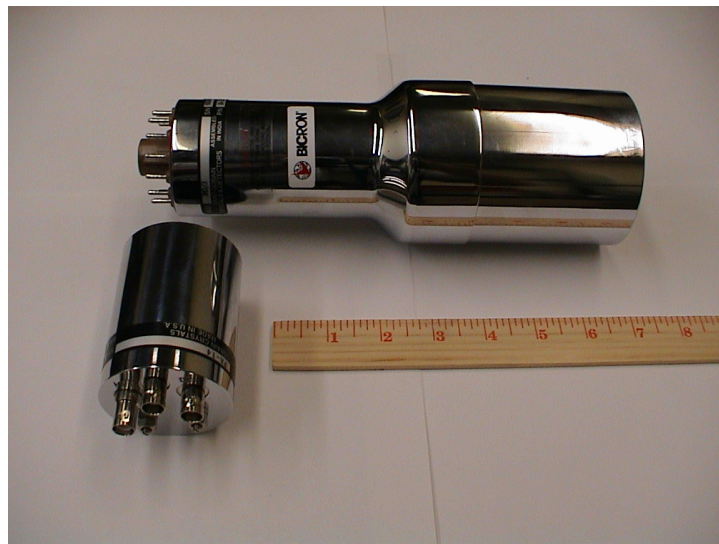
Figure 67. Photograph of NaI(Tl) detector
