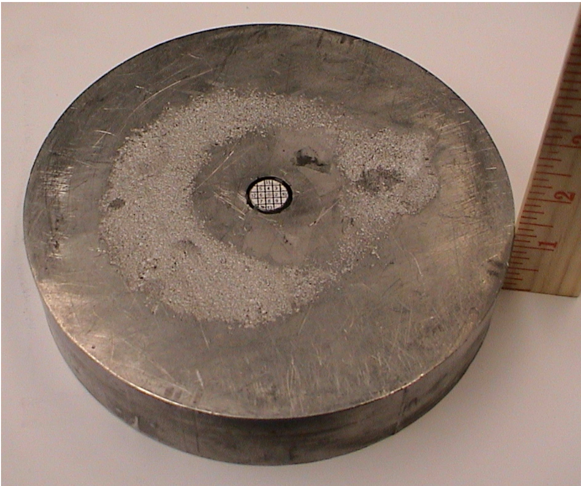
Figure 73. Photograph of conical collimator with alignment grid in center
