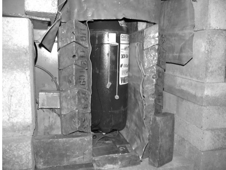
Figure 19. N 2 O in place at end of OSU beam port.
