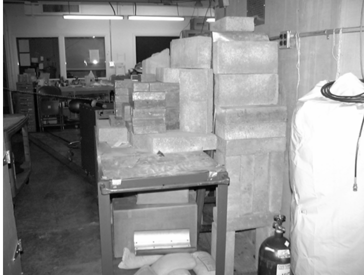
Figure 18. Shielding on end of OSU beam port.
