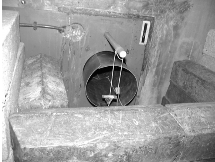
Figure 16. Characterization foils at end of beam port.
