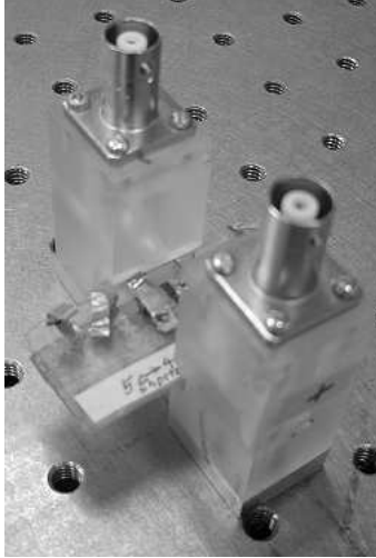
Figure 4.7: Single-stage device mount with device 2.
