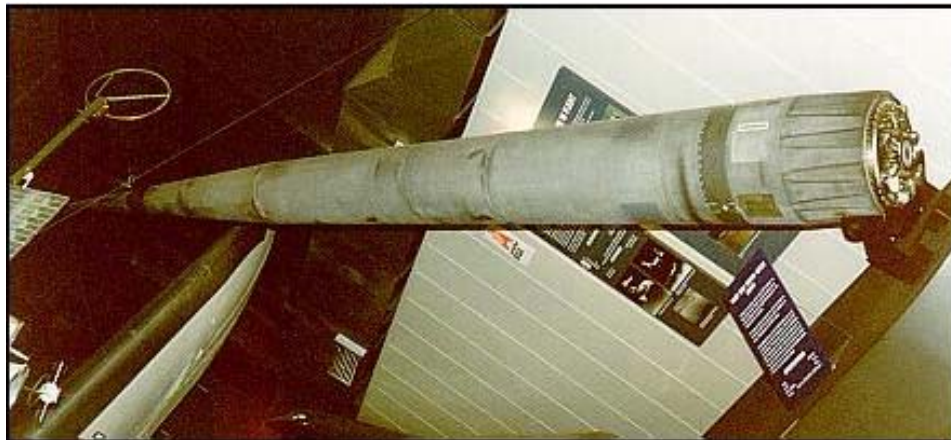
Figure 1-4: The Boost Glide Re-entry Vehicle investigated related technological problems, particularly hypersonic maneuvering after re-entry into the atmosphere. The test was flown on 26 February 1968 from Vandenberg AFB, California to the area of Wake Island in the Pacific Ocean.
