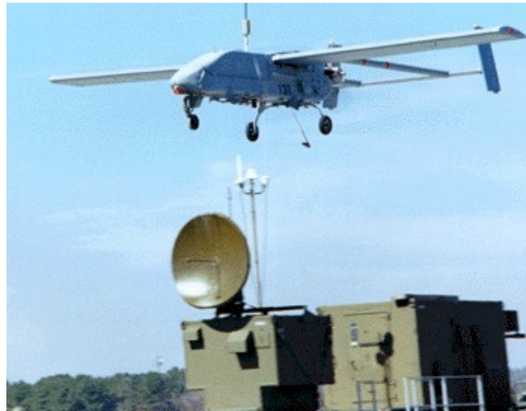
Figure 2.3 RQ-2A Pioneer UAV [36]
