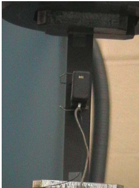
Figure 99. Elevation view of the test setup for tensile testing with extensometer
