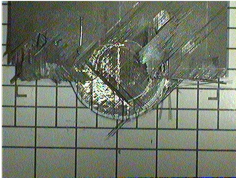
Figure 92. Back view of the top half of panel 418T after failure
