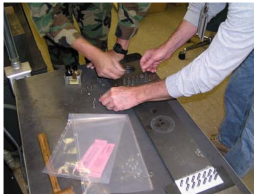
Figure 18. Large tensile specimens being bolted into the test fixture
