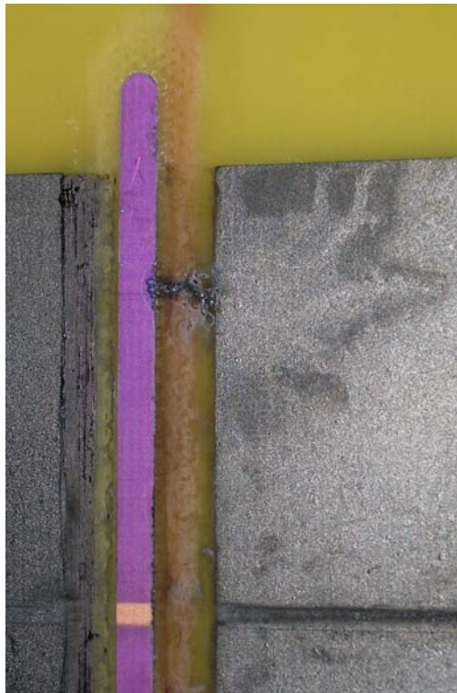
Figure 36. Arcing on an FR4 plasma actuator.
