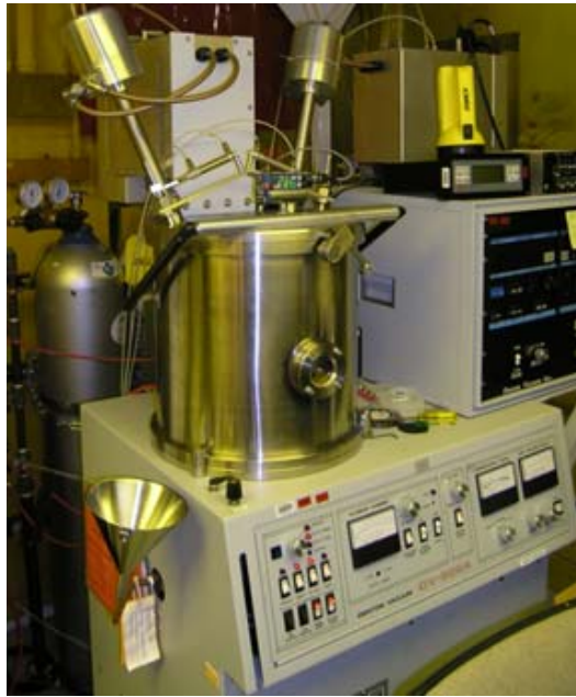
Figure 12. Denton RF magnetron sputtering system.
