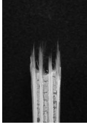
Figure 74. Creep Fracture Surface of N610/Mon/Alumina at 1100°C, 80 MPa (Side)
