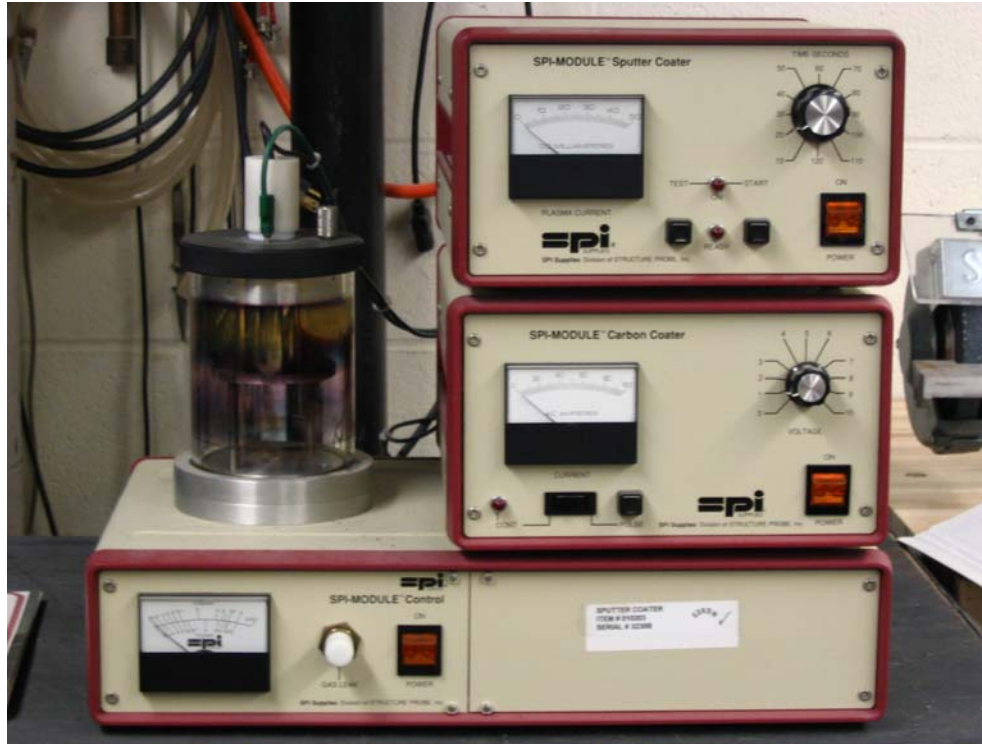
Figure 21. SPI MODULE Sputter Coater
