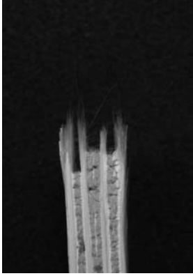
Figure 73. Creep Fracture Surface of N610/Mon/Alumina at 1100°C, 40 MPa (Side)
