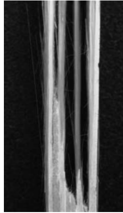
Figure 42. Tensile Fracture Surface of N610/Mon/Alumina at 1100°C (Side)
