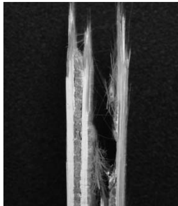
Figure 85. Creep Fracture Surface of N610/Mon/Alumina at 900°C, 120 MPa (Side)
