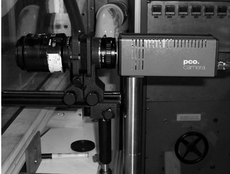
Figure 3.16: High speed digital camera used with PIV.
