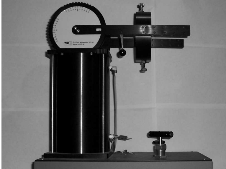
Figure 3.19: Apparatus used to calibrate a hot film anemometer.
