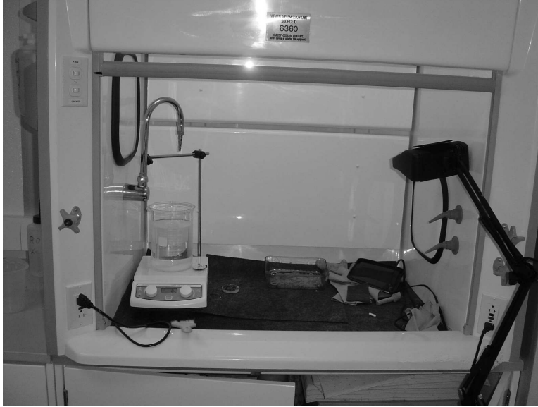
Figure 3.10: Vent hood used while etching copper.
