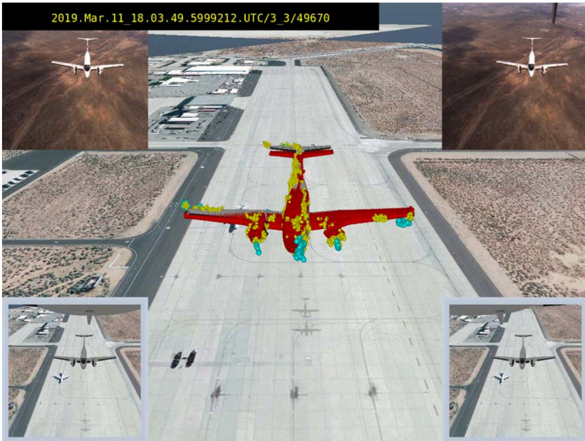
Figure 12: Calculated Relative Pose Estimations
