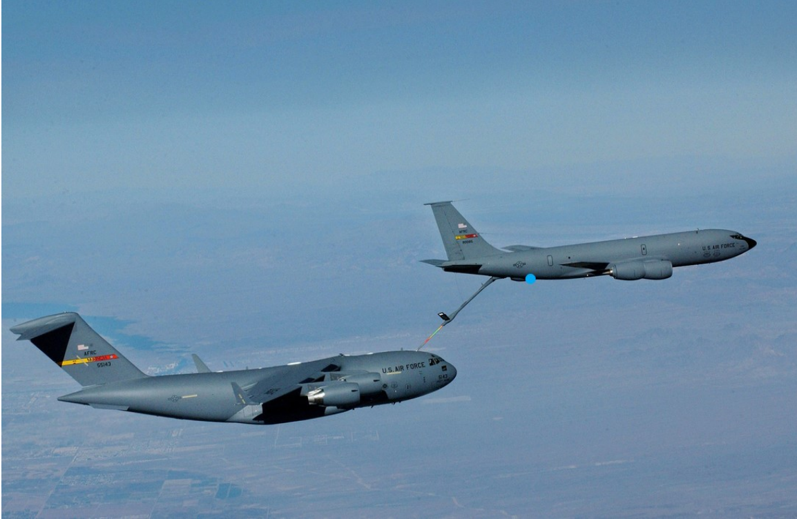
Figure 1: Aerial Refueling via Boom Method [1]
