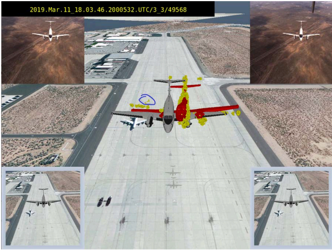
Figure 28: Relative Pose Estimation With Indicated Outliers
