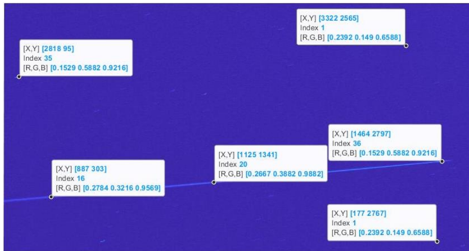
Figure 14a. Image of the upper portion of the beam taken with a G9 Canon digital camera. Pixel index and location are plotted along the beam to show the increase in brightness values at larger phase angles, indicating an increase in scattered irradiance.
