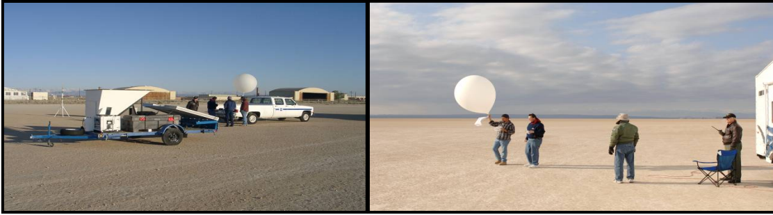
Figure 68. SODAR Equipment and Weather Balloon
