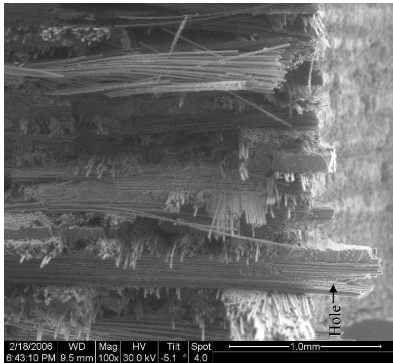
Figure 73. Specimen FH5 (notched, 175 MPa fatigue, 1200°C), 100x (hole along right side of image)
