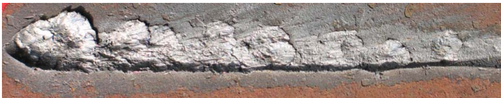
Figure 21 – Experimental Test 2 Gouge
