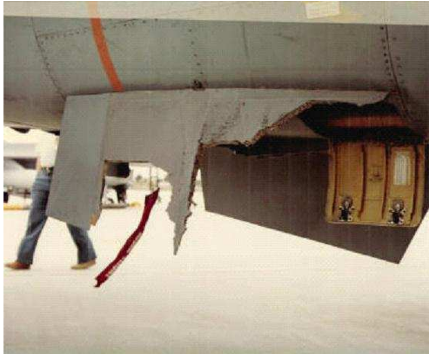
Figure 1.2: Ventral Fin Failure
