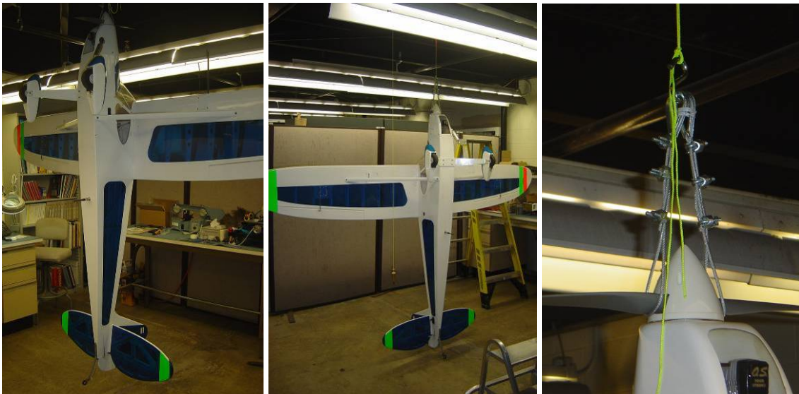
Figure 15. a) Inertia Test Set Up, b) Reverse View, and c) Wire Harness Apparatus
